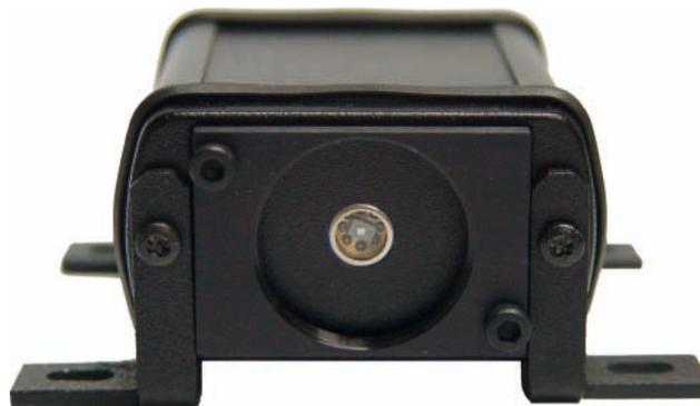
Figure 2. Single photon detector module: id100
