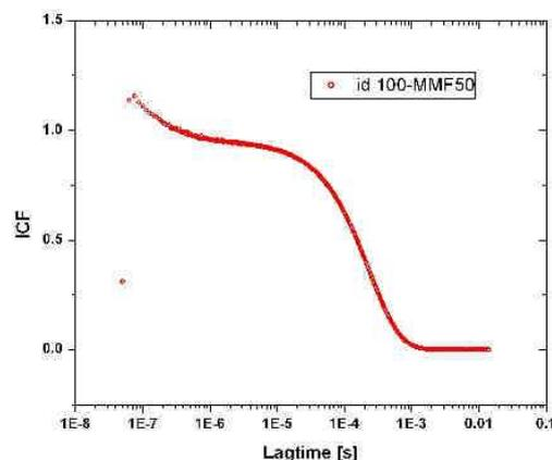
**Figure 2: Intensity correlation function (ICF) dependence with time, in auto-correlation measurement. Courtesy of LS Instruments.**
