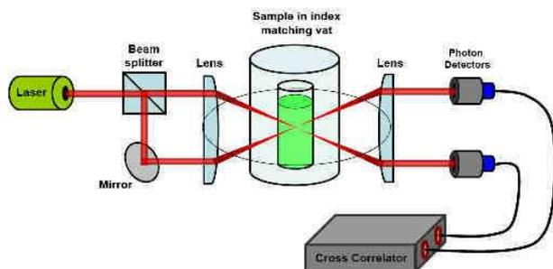
**Figure 3: Cross-correlation experimental setup. Courtesy of LS Instruments<sup>1</sup>.**
