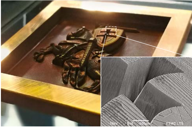
3D milled sample in copper. Zoom in SEM image.
