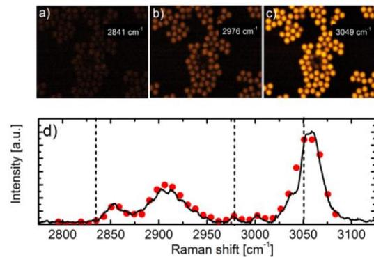
Figure 4. Demonstration of a multicolor SRS measurement of polystyrene beads. The system was tuned from  $2750\text{ cm}^{-1}$  to  $3150\text{ cm}^{-1}$  with the fast sweep function. The recorded data (red dots) is in perfect agreement with the theoretical data (solid line). Images a), b) and c) show three different images of the scan.
