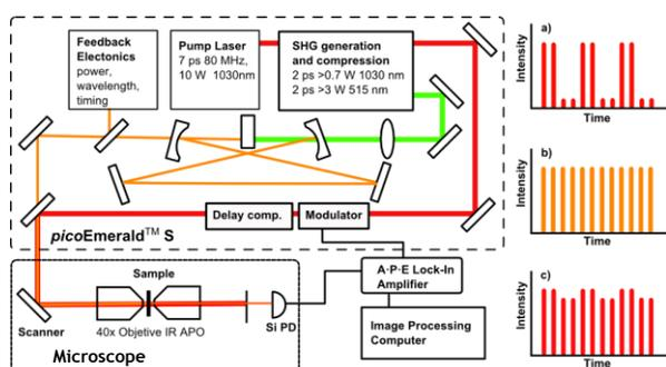
Figure 1: Schematic setup of the *picoEmerald™ S* and the used setup for the comparison measurements. The pump laser, SHG, OPO, and electronics are all in one housing (dotted line) and provide co-propagating Pump and Signal beams with synchronized pulses.
