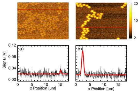
Figure 3: Two images of polystyrene beads ( $1\mu\text{m}$ ) in water recorded with a standard light source and 7 ps pulse duration (left) and one recorded with the new *picoEmerald™ S*. The line data taken from the above images in the bottom graphs allows quantifying the improved Signal-to-Noise ratio.
