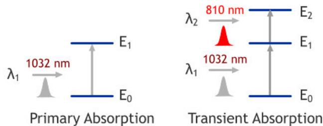
*Energy Diagrams of the transient absorption principle (wavelength numbers are only examples).*
